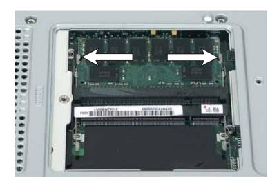
**9** Pull the memory module out of the slot.
